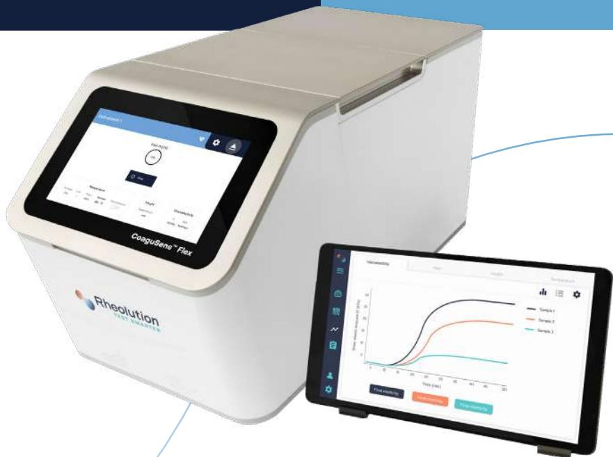
**CoaguSens™ Flex is a benchtop instrument that precisely characterizes in real-time, without contact and without destroying the sample, the viscoelastic properties of milk gel during coagulation. Samples are contained into removable sample holders that can be disconnected, stored out of the instrument and re-connected for re-testing as many times as required.**
