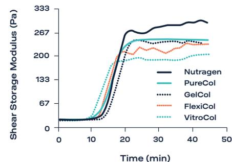
Fig. 3: Gelation kinetics of Nutragen® (6 mg/mL), PureCol® (3 mg/ml), GelCol® (3 mg/mL), FlexiCol® (3 mg/ml), and VitroCol® (3 mg/ml) at 37 °C.
