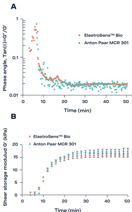
Fig. 1: Comparison of ElastoSens™ Bio and rotational rheometer measurements during the formation of agar gel: (A) comparison of the phase angle; (B) comparison of the shear storage modulus.
