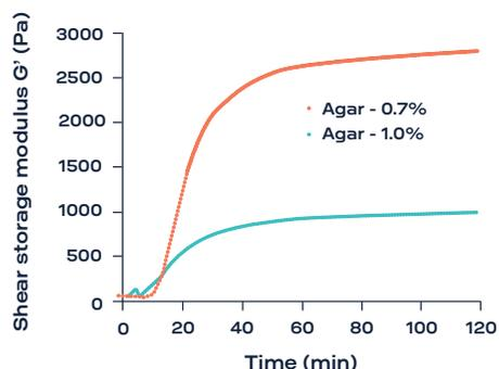
Fig. 2: Time evolution of the storage shear modulus ( $G'$ ) during the formation of two agar hydrogels with different concentrations (0.7 % and 1.0 %, w/w)
